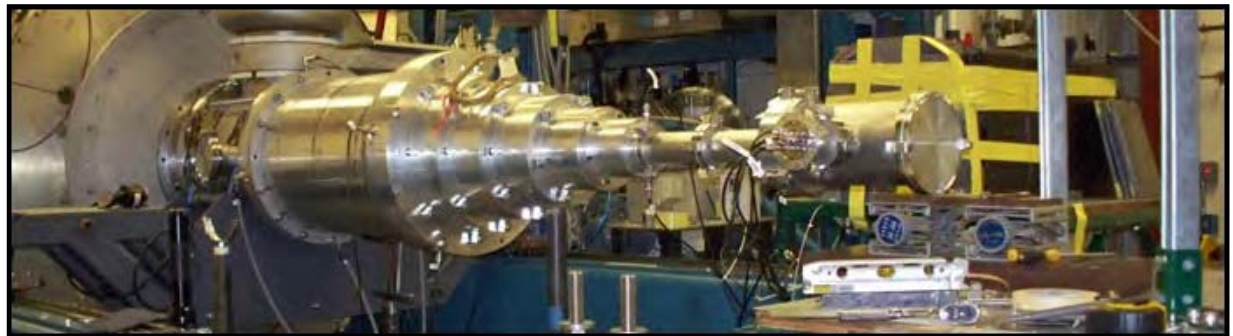
Investigation of power flow in radiographic diodes using 8 MV, 200 kA, 50-ns "Mercury" pulsed power generator
